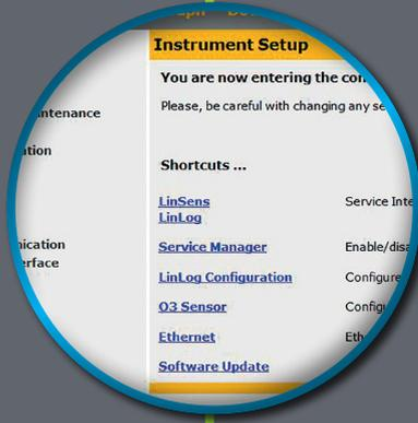
The airQrate is equipped with a powerful logger functionality (based on recordum airQlog). Thus, the devices' current measurement values can be recorded and analysed synchronously with the calibration system's nominal values.
