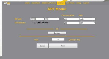
Start the calibrations on the internal touch screen.
